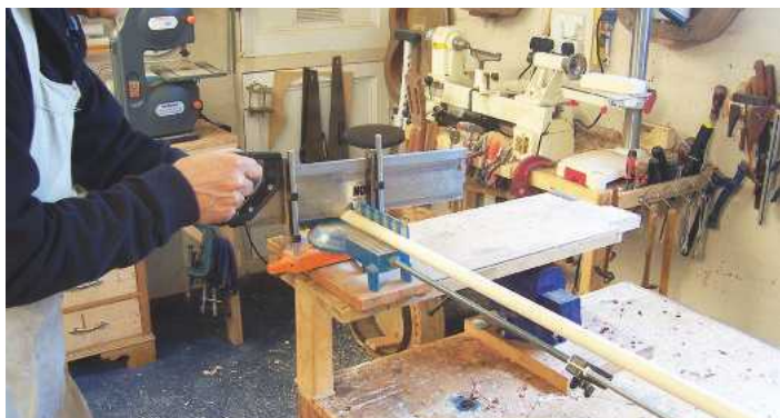
▲ Pic.7 Shaun modified his old Nobex mitre cutter by making a longer depth stop from threaded bar before cutting the dowels at right angles
